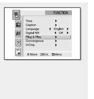
Note: Plug & Play feature doesn't work when the V-chip is on or when in the A/V mode.
